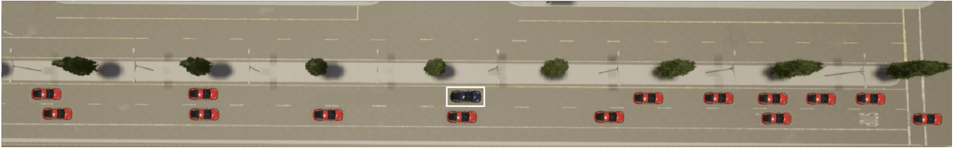
Fig. 5. A screenshot of one of the CARLA simulator scenarios is shown, where the ego-car is the blue car in the white rectangle. In this scenario, the ego-lane is randomly blocked and the ego-car is required to perform a lane change.
